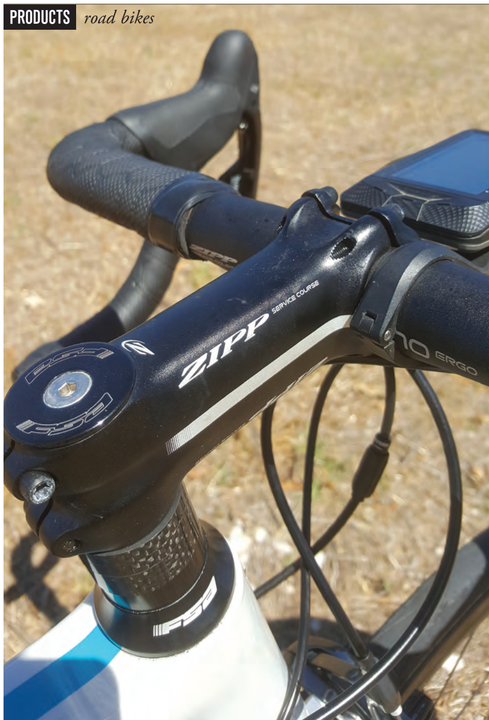
▲ Zipp's aluminium Service Course bars and stem are fast becoming a favourite; light and stiff, without the carbon scare factor.
